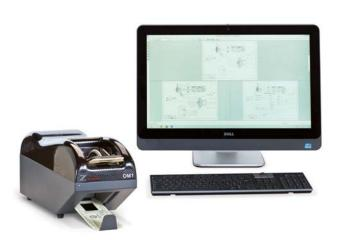
The OM 1 is a compact aperture card scanner. It creates digital images from microfilm aperture cards that can be instantly accessed, searched, viewed, printed or emailed. The OM 1 comes with Hollerith read and auto-feed hopper, for unattended batch scanning. Simple operation makes this scanner an ideal digital alternative to reader-printers.
